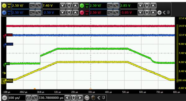
TXD =  $V_{CC1}$        $R_L = 60\ \Omega$        $V_{CC1} = V_{CC2} = 5\text{ V}$
