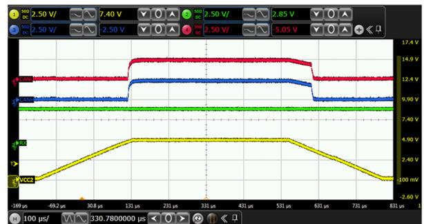
TXD =  $V_{CC1}$        $R_L = 60\ \Omega$        $V_{CC1} = V_{CC2} = 5\text{ V}$
